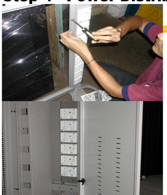
In the power distribution is placed on bottom of the rear main frame
