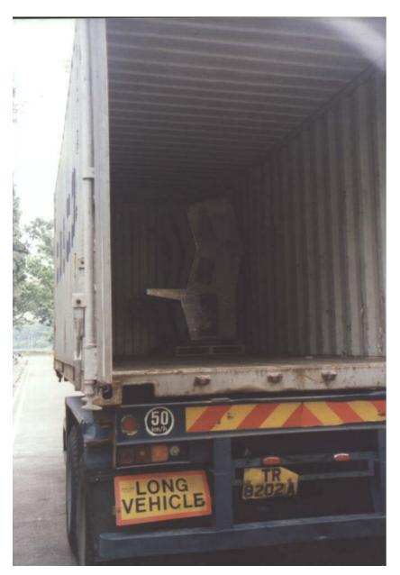
• As the container will be subjected to shock and vibration, every bay is spaced to prevent knocking between console during transport stage.
