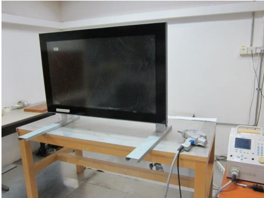
Electrostatic Discharge Immunity Test Setup
