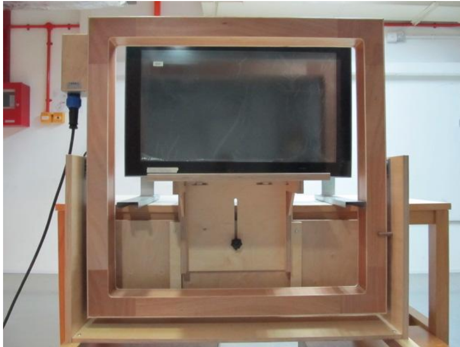
Power Frequency Magnetic Field Immunity Test Setup
