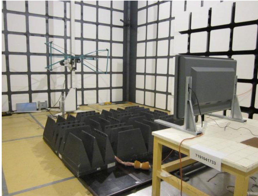
RF Radiated Immunity Test Setup
